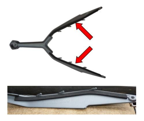
Apply both foam strings inside the "Y shape" cover just below the hooks
