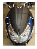
Remove the pointed 9 screws and take off the dashboard cover
