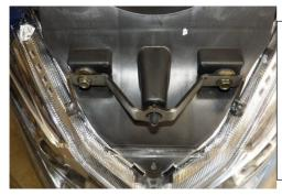
Using the original bolts and washers, center and fix the provided bracket and welded bushes in up position; put on again the dashboard cover and fix it
