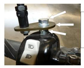
Fit the mirrors using the provided spacers, plates, washers and m8 bolts
