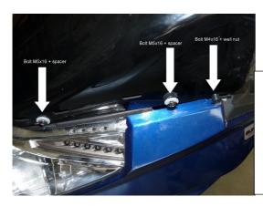
Fix the windshield using bush and screw M5x16 for the front fixation, bush and screw M5x16 for the rear and the well nut in the hole
