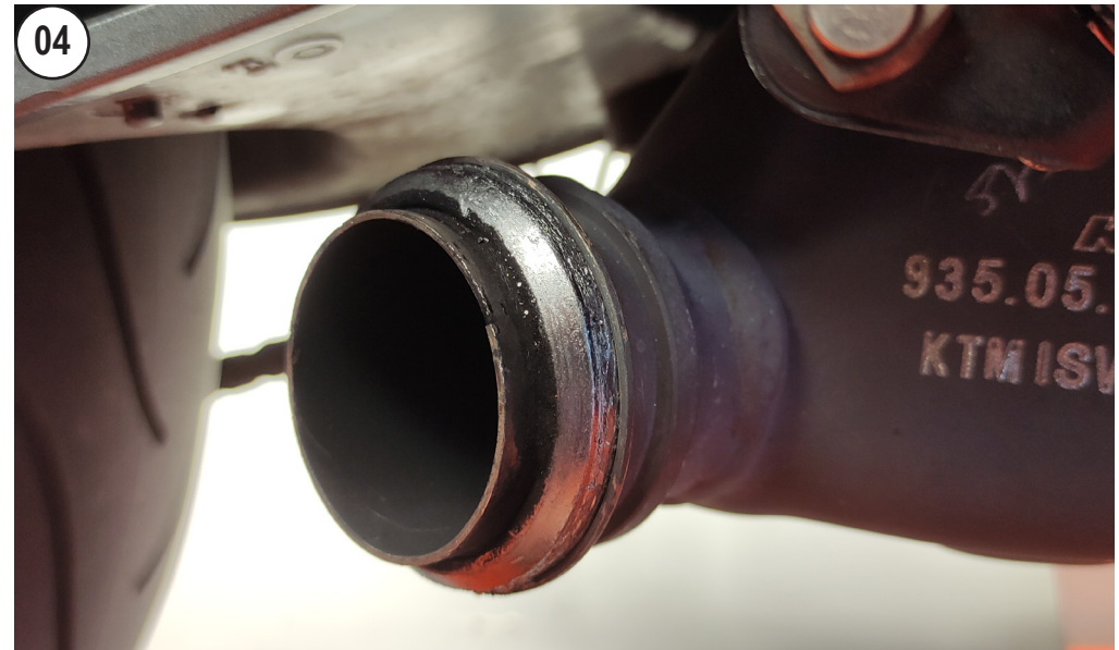
REMOVE THE STOCK PIPE - USE ORIGINAL BUSHING OR REPLICE WITH A NEW ONE
