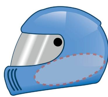
2. The surface of each part must be **minimum 18 cm<sup>2</sup>**.
